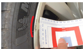
Charges applicable to over 50mm. Image 2 shows 40mm which is within tolerance.
